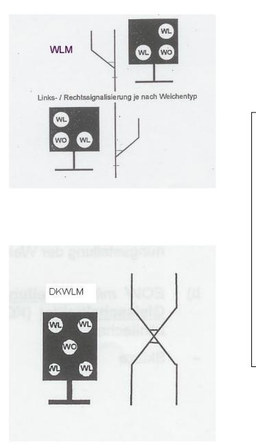
The points position indicator PPI / double crossing points position indicator DCPPI consists of: POI = points orientation indicator PPI = points position indicator
