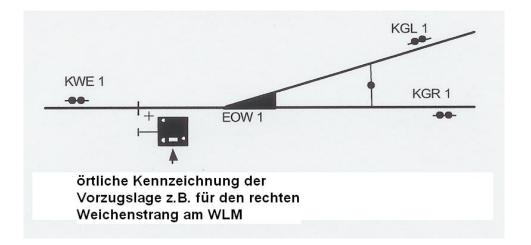
In the image above: CPE, ELP, CTL (Crossing Track Left), CTR (Crossing Track Right) Local identification of the priority position, for example, for the right-hand points branch of the PPI
